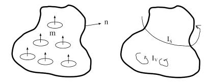
Elementary current will tend to cancel on the inside. If the cancellation is complete, then there will only be a surface current (Units:  $Am^{-1}$ ). If not complete, then there will be a volumetric current density (Units:  $Am^{-2}$ ).
