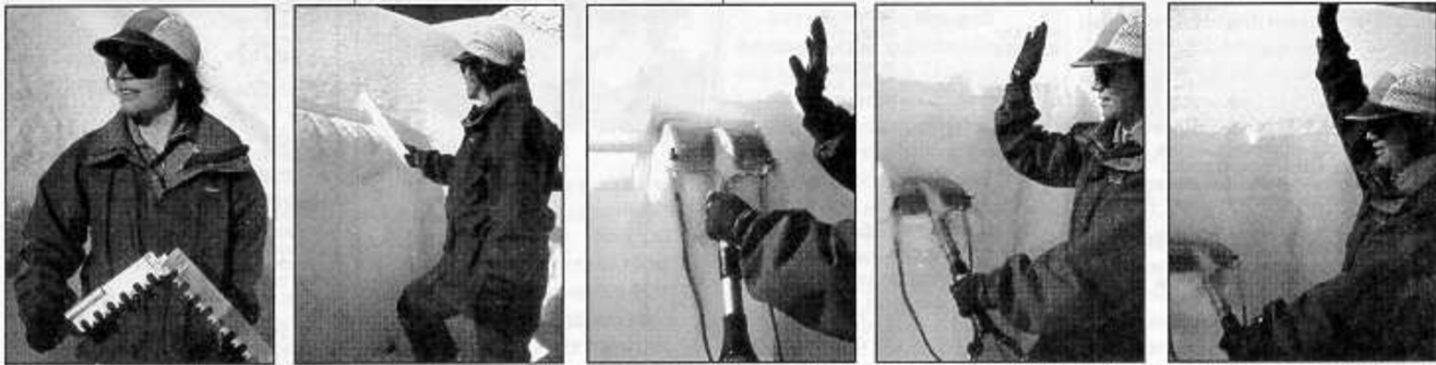
Compression Test — Using a lightweight saw, make vertical cuts in the back snowpit wall about the same width your shovel blade. Then cut the back of the column with the snow saw so the column is completely isolated. Lay the shovel blade on top of the column and tap gently articulating from the wrist. Then tap progressively harder articulating from the elbow, then finally very hard articulating from the shoulder. Do several of these tests to get a representative sample.
