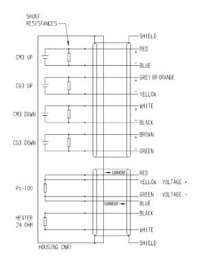
FIGURE 5-1. CNR1 Schematic
