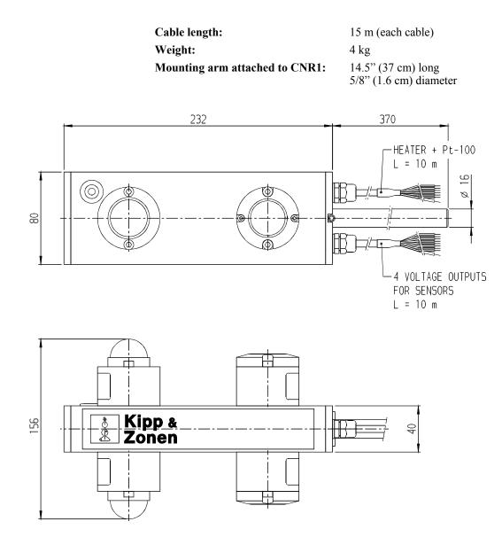
FIGURE 2-1. The Dimensions of the CNR1
