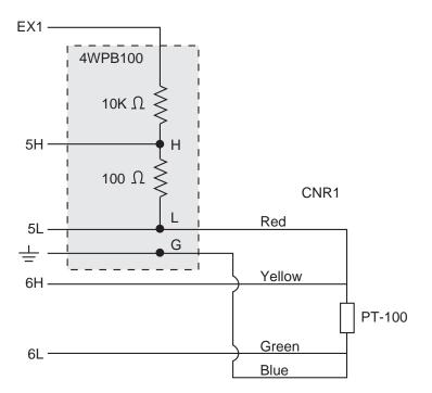
FIGURE 5-2. Interfacing the Pt-100 Using the 4WPB100 Module
