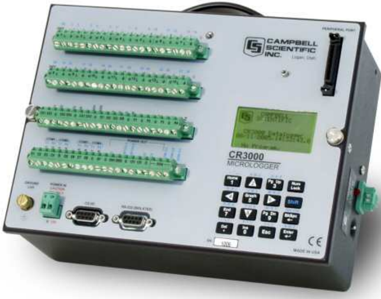
FIGURE 1.10-1. CR3000 with wiring panel.
