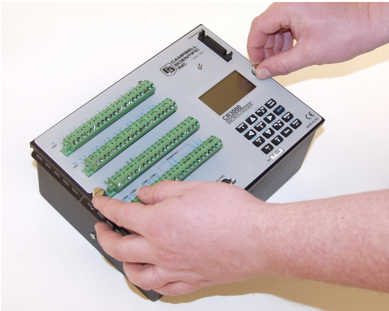
FIGURE 1.10-2. Loosen thumbscrews to remove CR3000 wiring panel from base.
