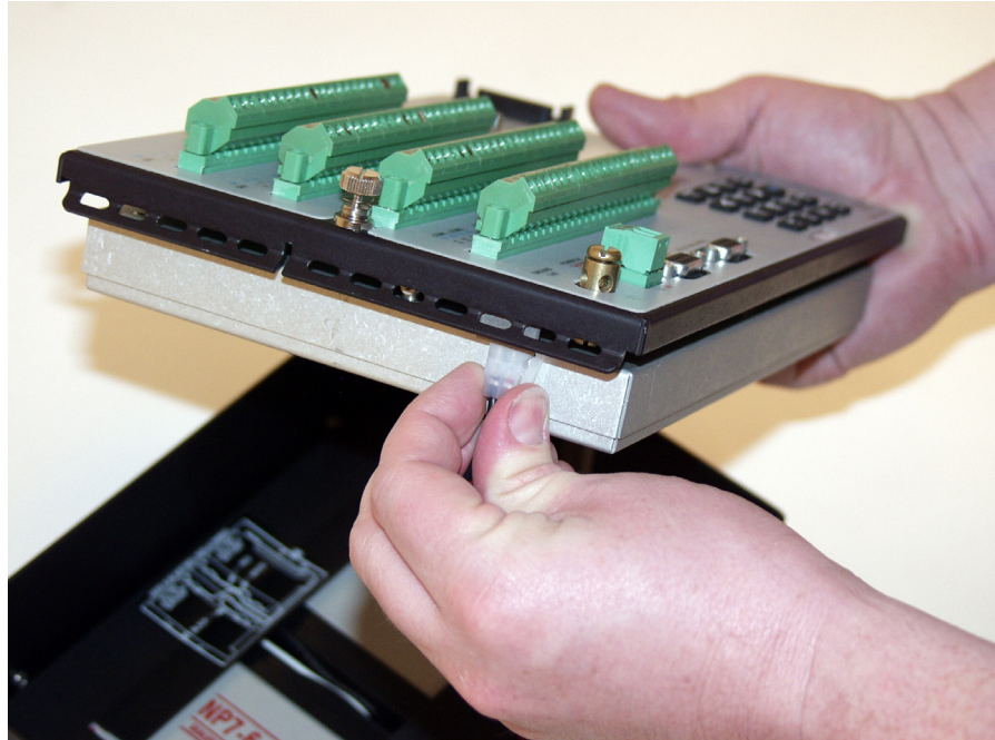
FIGURE 1.10-3. Disconnect internal battery from wiring panel (BPALK and Sealed Rechargeable base only).
