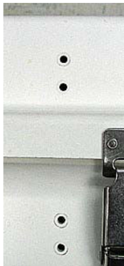
FIGURE A.1-2. The proper placement of the screw holes are shown in a close-up (left photo) and distant view. Ensure that the screw holes for both brackets are aligned with each other.
