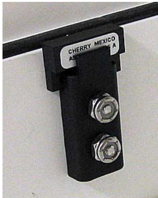
FIGURE A.1-4. Actuator installed in the enclosure door.
