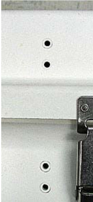
FIGURE A.1-11. The proper placement of the screw holes are shown. Ensure both brackets are aligned with each other.
