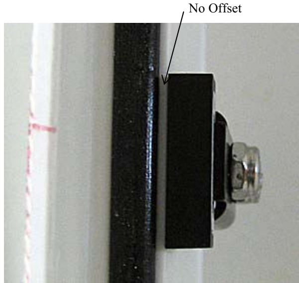
FIGURE A.1-1. This procedure is for ENC16/18 enclosures that do NOT have an offset near the edge of the enclosure door. Follow the procedure provided in section A.1.2 if your ENC16/18 has an offset.
