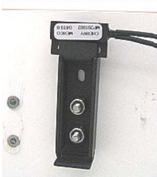
FIGURE A.1-9. The switch mounts inside the enclosure case. Line up the switch so that the screws fit in the holes previously drilled.
