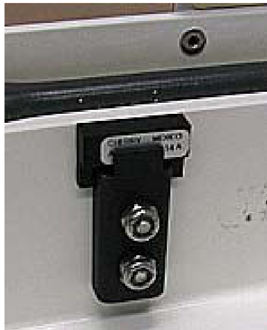
FIGURE A.1-10. The actuator mounts inside the enclosure lid. Line up the actuator so that the screws fit in the holes previously drilled.
