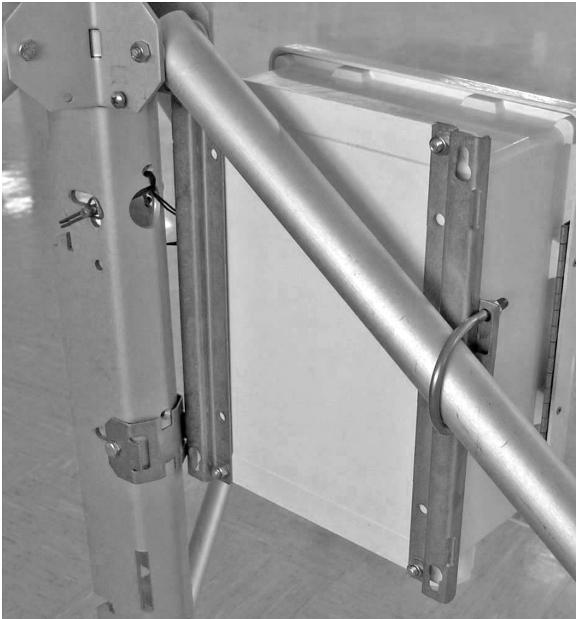
FIGURE 4-10. An enclosure attached to the leg base of a CM110 tripod.
