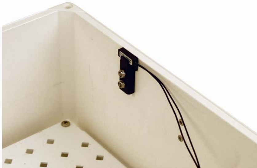
FIGURE A.1-15. The switch attached to the enclosure case.
