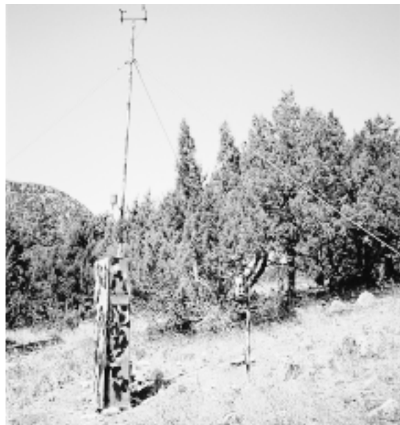
This station is camouflaged to prevent "human pests" from damaging the station.
