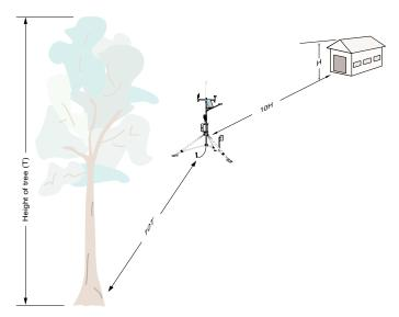
Wind sensors should be located over open level terrain. The EPA recommends the wind sensor be a distance of at least ten times the height of nearby buildings, trees, or other obstructions.
