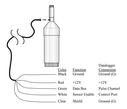
FIGURE 3. Pulse Train Wiring
