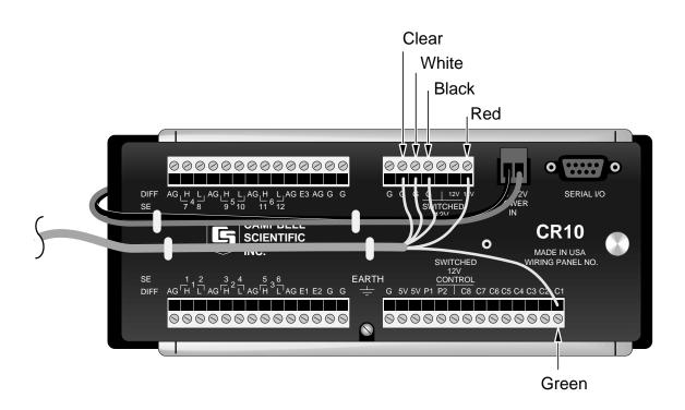
FIGURE 2. SR50 Wiring for CR10(X) SDI-12 Example
