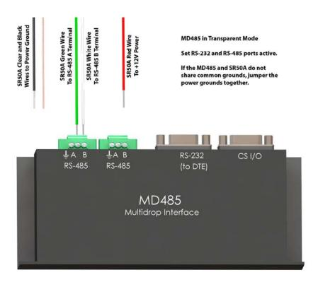
FIGURE 1. SR50A to MD485 Wiring
