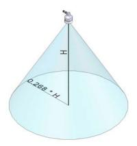
FIGURE 2. Beam Angle Clearance
