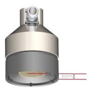
FIGURE 3. Distance from Edge of Transducer Housing to Grill
