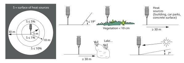
Figure 1.B.2. Criteria for air temperature and humidity for class 2 sites
