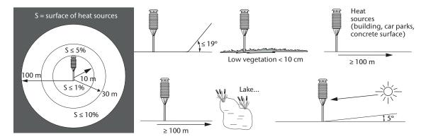
Figure 1.B.1. Criteria for air temperature and humidity for class 1 sites
