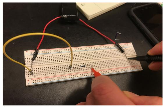
• Measuring the current on one side of the resistor; note that the prongs of the multimeter complete the circuit (i.e. orange male-to-male wire was removed). The dial should be set to the "mA" setting.
