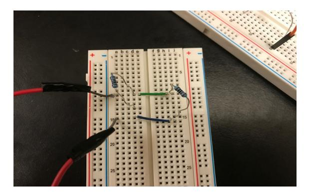
• Note that the bottom leg of the leftmost resistor was moved so that it's no longer in the same row as the blue jumper wire and the other end of the battery. You can measure the current at B by connecting the multimeter between the bottom leg and the blue wire.
