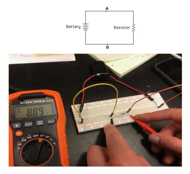
• Measuring the voltage across the resistor. The circuit is completed with the male-to-male wires. Note that the prongs of the multimeter are in contact with both legs of the resistor. The dial should be set to the "V" setting.
