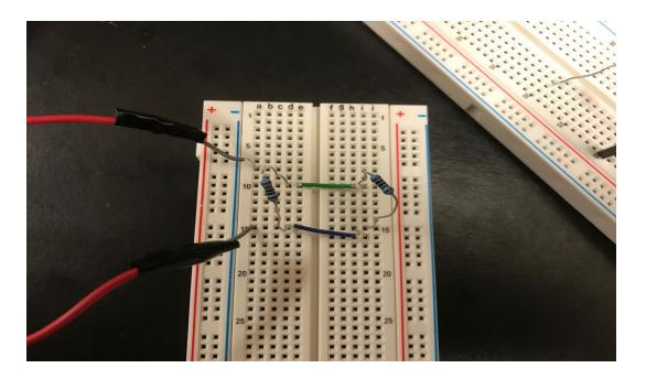
• Note that the top battery wire was moved so that it's no longer in the same row as the leftmost resistor; the circuit is broken. You can then measure the current at A by connecting the multimeter prongs in series between the battery and the left resistor.
