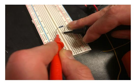
• Measuring the resistance of a resistor. The dial on the multimeter should be set to the Ω setting. Note that the resistor is not part of any circuit (the multimeter itself provides the voltage across the resistor).
