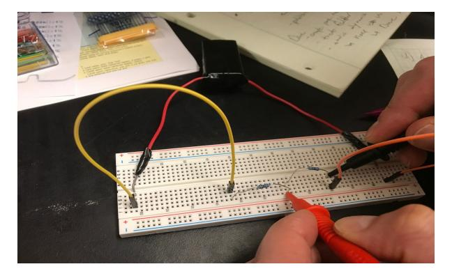
• Measuring the voltage across one resistor. The circuit is completed with the male-to-male wires. Note that the prongs of the multimeter are in contact with both legs of the resistor. The dial should be set to the "V" setting.
