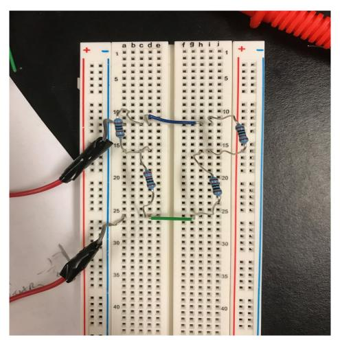
• Bridge circuit, completed. Note that the bottom left resistor should be the unknown (**Green**) resistor.
