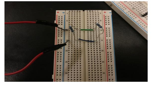
• Note that the bottom leg of the rightmost resistor was moved so that it's no longer in the same row as the blue jumper wire. You can measure the current at C by connecting the multimeter between the bottom leg of the rightmost resistor and the blue wire.
