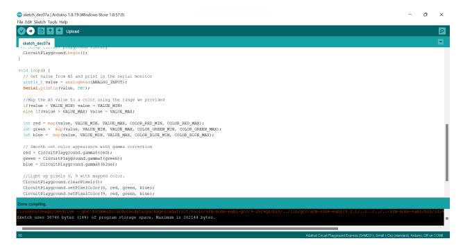
We will also open up the serial monitor while we wait for it to upload. **Tools->Serial Monitor** or **CTL-SHIFT-M**
