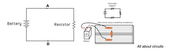
Imagine you connected the battery in series with a  $1k\Omega$  resistor (similar to the left figure above).
