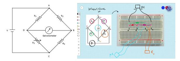
Imagine you connected three known and one unknown resistor (**Green**) in a bridge circuit (as shown in the left figure above).
