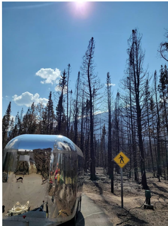
Figure 54: Minor damage to aluminum clad trailer that was surrounded by full canopy consumption crown fire in mature trees.
