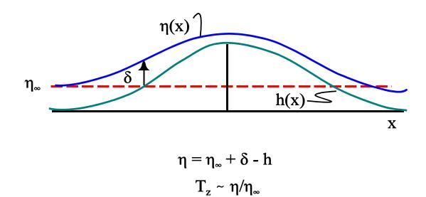
Figure 2-27. Depiction of streamline height ( $\eta$ ), streamline deflection ( $\delta$ ), and strain factor ( $T_z$ ) nomenclature.
