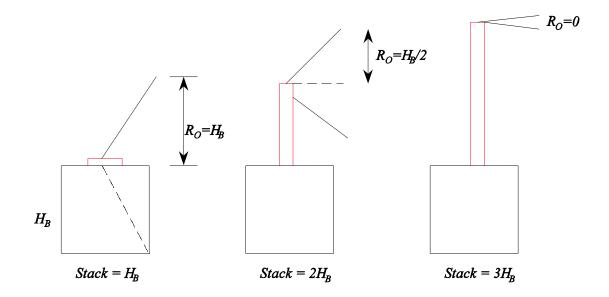
Figure 2-11. Illustration of the initial dilution radius, R<sub>o</sub>, as a function of stack height for a squat building (From Schulman and Scire, 1981). Momentum plume rise is neglected in the figure.
