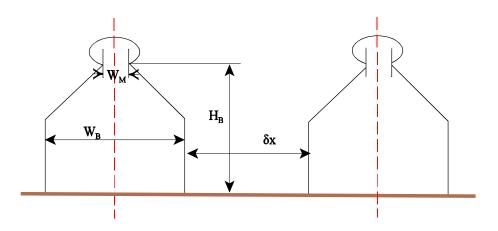
Figure 2-35. Cross-section of adjacent buildings with dimensions defined for BLP (from Schulman and Scire, (1980)).
