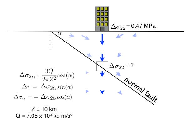
these equations assume z is positive downward, so Q is acting in the +z direction
