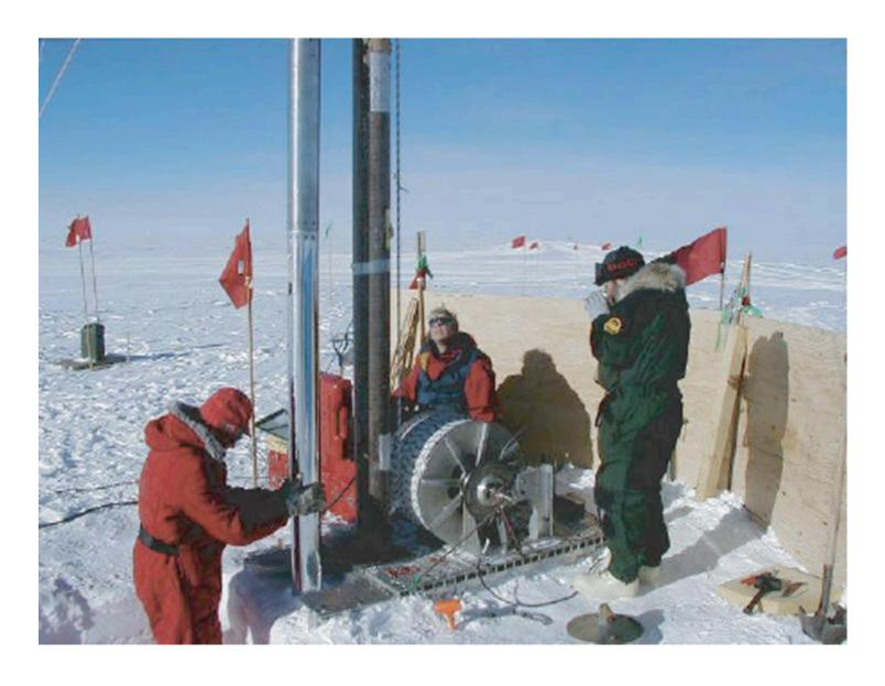
> some sites involve seismometers in boreholes to minimize noise
