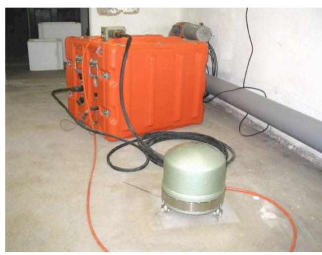
A modern **seismograph** records ground motion (from a seismometer) in digital format onto magnetic or optical disk
