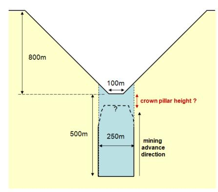
The open pit is approximately 800 m deep and 100 m wide at the bottom with  $45^{\circ}$  slopes. Exploration drilling indicates that the ore body is vertical, 250 m wide (centred with the pit floor bottom) and continues to depths of more than several hundred metres below the pit bottom. Plans are to sink a 1300m deep shaft, and to mine the ore body upwards until reaching the bottom of the crown pillar (which is for you to determine).
