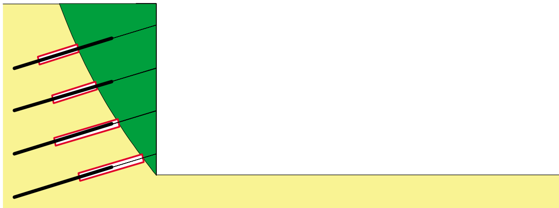
Fig. 20. Inclusion of pile embedment resistance in a limit equilibrium analysis.
