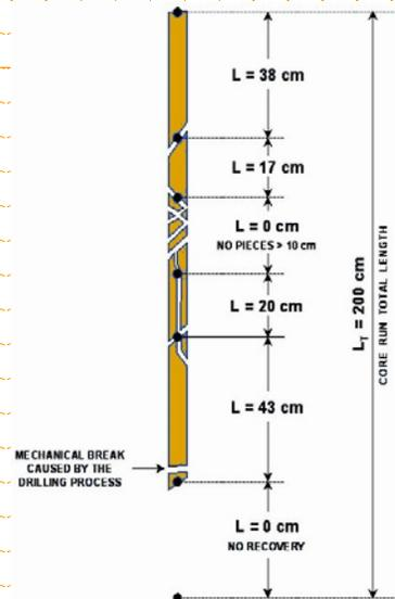
$$RQD = \frac{\sum \text{Rock Pieces} \geq 10 \text{ cm}}{\text{Core Run Total Length}} \times 100 (\%)$$
