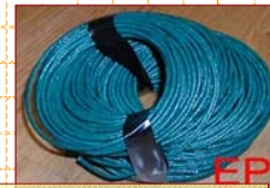
Safety fuse: Gives miner time to light all fuses and still have time to seek safety before the blast occurs.
