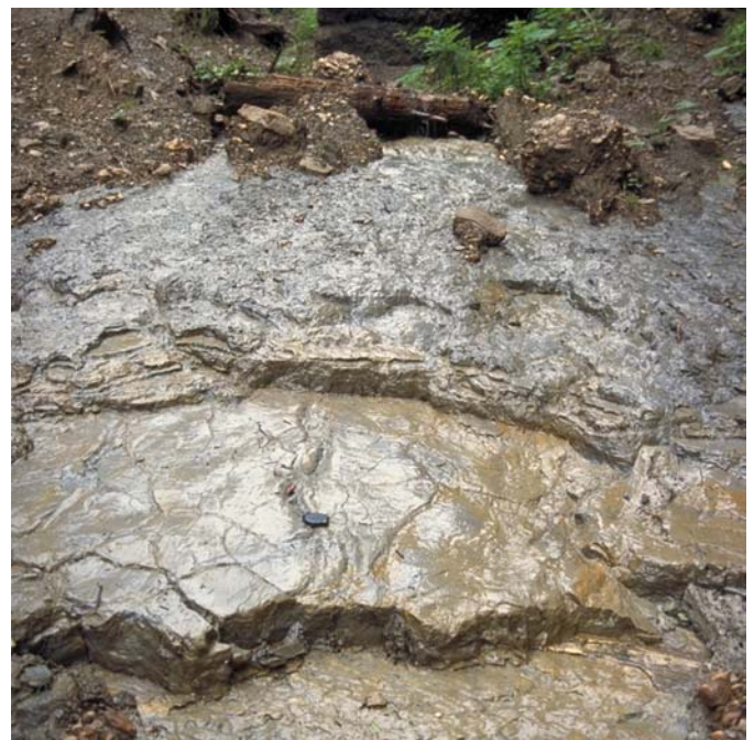
Figure 9. Upper Rufi slide surface through marl layers.
