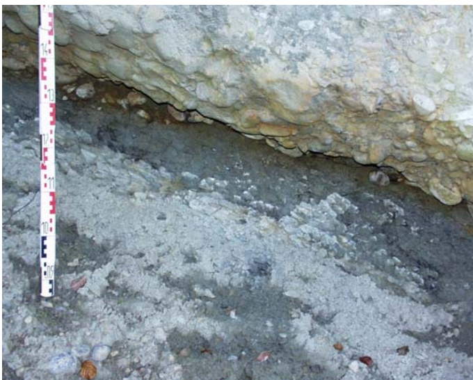
Figure 11. Conglomerate block overlying weakened weathered marl.
