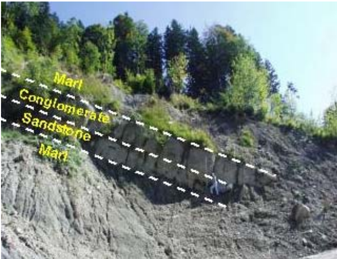
Figure 5. Bedding sequence of the interbedded conglomerates and marls along the margin of the Rufi slide.
