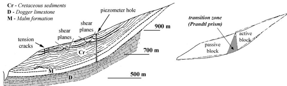
Figure 4. Schematic cross-section of the Vaiont slide showing transitory damage zone development in the form of a Prandtl prism (after Mencl 1966)
