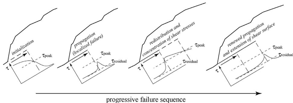
Figure 1. Shear surface development by progressive failure (after Bjerrum 1967)
