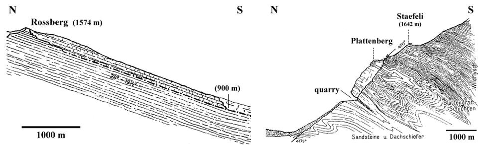
Figure 3. Schematic cross-sections of the Goldau (LEFT) and Elm (RIGHT) rockslides (after Heim 1932)
