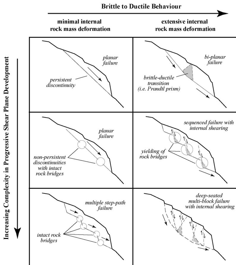
Figure 2. Massive rock slope sliding mechanisms as controlled by progressive shear plane development and internal rock mass deformation/damage
