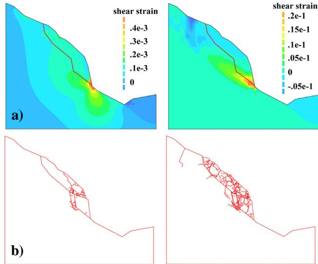
Figure 7. Numerical modelling of progressive shear plane development through: (a) continuum techniques showing shear strain development during cohesion loss; (b) hybrid continuum/discontinuum techniques showing evolution of brittle fracture network development (after Eberhardt et al. 2002)
