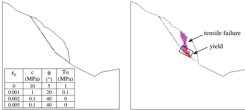
Figure 8. Distinct-element strain-softening model showing development of Prandtl yield zone at base of slide surface and propagation of tensile damage upwards through intact slide mass, dividing the slide mass along the contact between first and second Randa rockslide events
