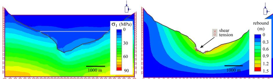
Figure 6. Finite-element continuum modelling of initial loading conditions due to glaciation (LEFT) and initiation at toe of Randa slope due to glacial rebound (RIGHT)
