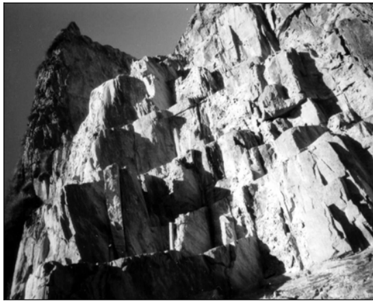
Figure 5. Back scarp of 1991 Randa rockslide showing limited nature of joint persistence and step-path configuration
