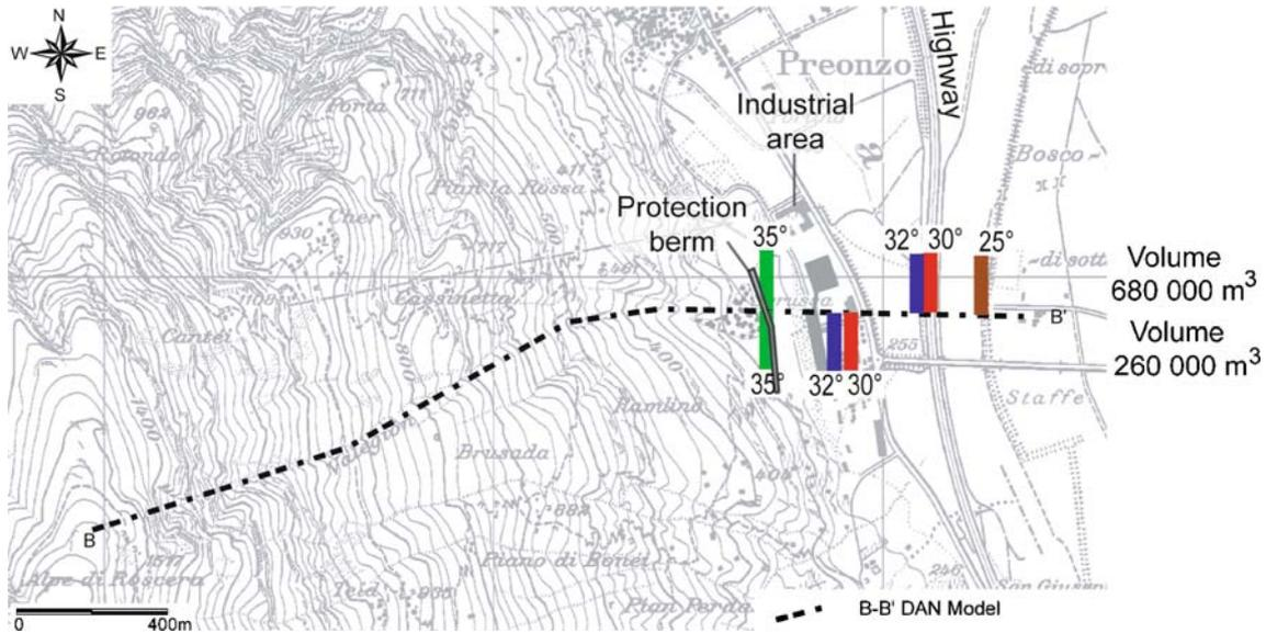
**Fig. 10** Maximum runout distances for the two different rock volumes in dependence of the friction angle of the underground. The analyzed travel path is indicated by the dotted line. Contour map is reproduced by permission of Swisstopo (BA091024)
