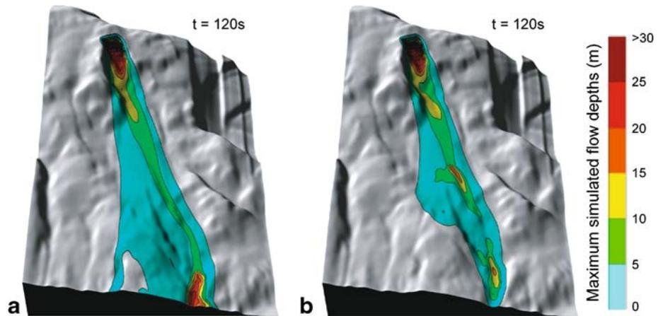
**Fig. 12** Maximum extent of the rockslide runout for the large rock volume in dependence of the channel width in the valley for constant friction angle of 30° on the slope and 20° in the valley. Contour map underlay is reproduced by permission of Swisstopo (BA091024)
