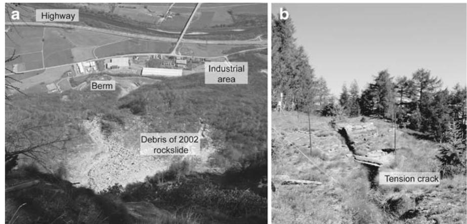
more to form step-paths of a deeper-seated rupture surface, continuum modeling has been shown to be sufficiently effective in providing an estimate of the depth of failure (Eberhardt 2008), especially when constrained by a tension crack at the top of the slope as in the case of Alpe di Roscioro.
