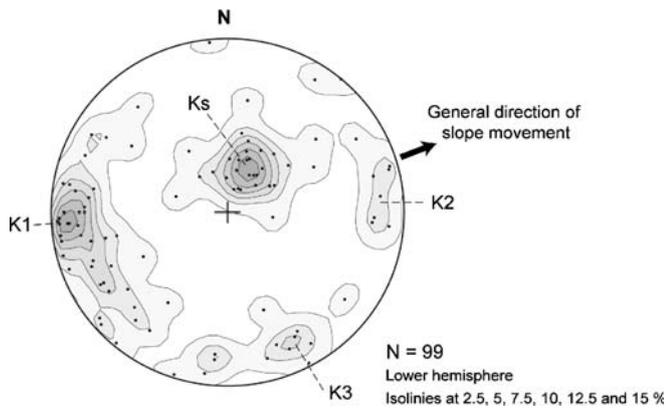
**Fig. 5** Fracture orientation distribution in a lower hemisphere projection. Fracture set  $K_s$  is oriented parallel to foliation and three steep fracture sets (K1-3) are present
