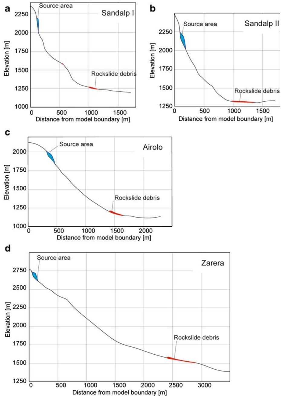
valley floor and is based on the authors' previous experience back-analyzing rock avalanches that impact wet alluvium. The results for these model runs, summarized in Fig. 12, show that even though the rockslide runout distance decreases with increasing spreading of the debris, the industrial area is still impacted in each case.
