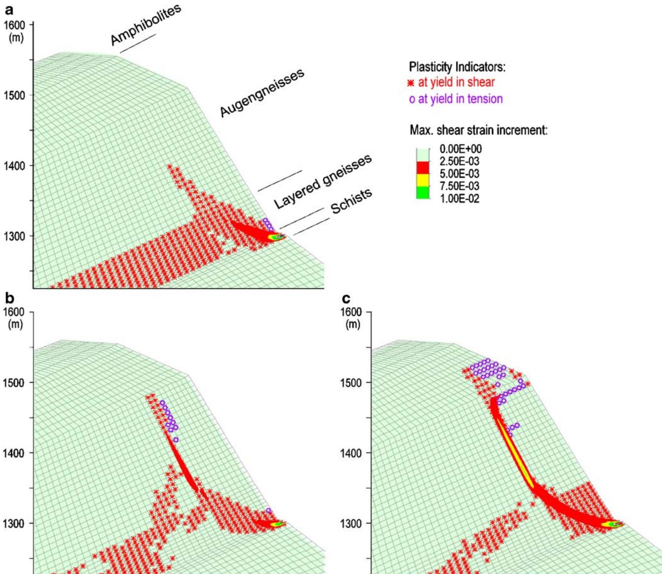
**Fig. 7** Numerical modeling results using the continuum-based finite-difference code FLAC
