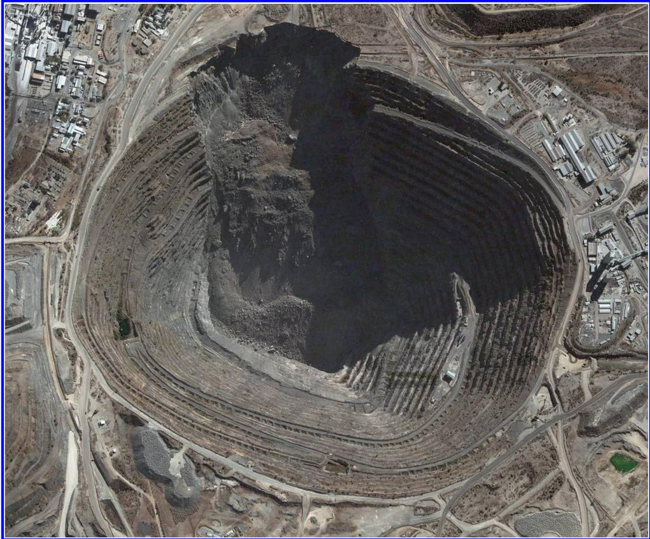
**1** Quickbird image of the Palabora mine in South Africa showing an example of a cave-pit interaction that led to the failure of an 800 m high pit slope
