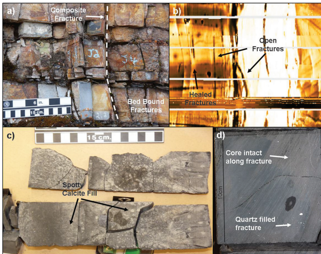
Fig. 1. Examples of natural fractures present in shales: (a) Devonian shale outcrop from northeastern British Columbia, (b) borehole image log from a horizontal well through the Muskwa – Otter Park formation, (c) open and partially open fractures in retrieved core, and (d) closed fractures in core samples from the Muskwa – Otter Park formation (after Reine and Dunphy 2011).
