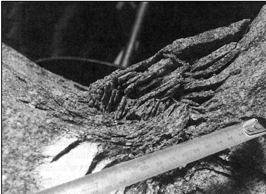
Figure 1.2 Development of thin slab failure zone through stress-induced brittle microfracturing (after Martin, 1997).
