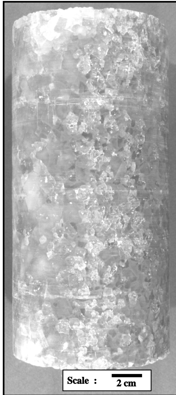
Figure 6.17 Coarse grained Saskatchewan potash sample prior to testing.
