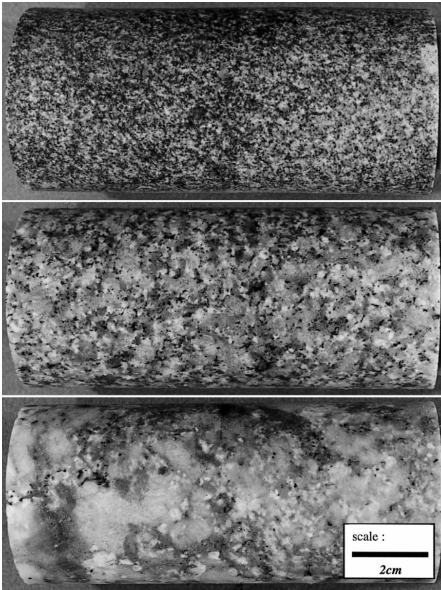
Fig. 3. Test samples from the 240 m level of the URL showing varying grain size: granodiorite (top), grey granite (middle), and pegmatite (bottom)
