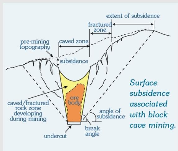
Eberhardt and colleagues at UBC, Simon Fraser University, and international partners Rio Tinto and Diavik Diamond Mines are studying the causal effect of geological faults and fractures on mining-induced subsidence patterns, and their effect on sensitive surface structures.
