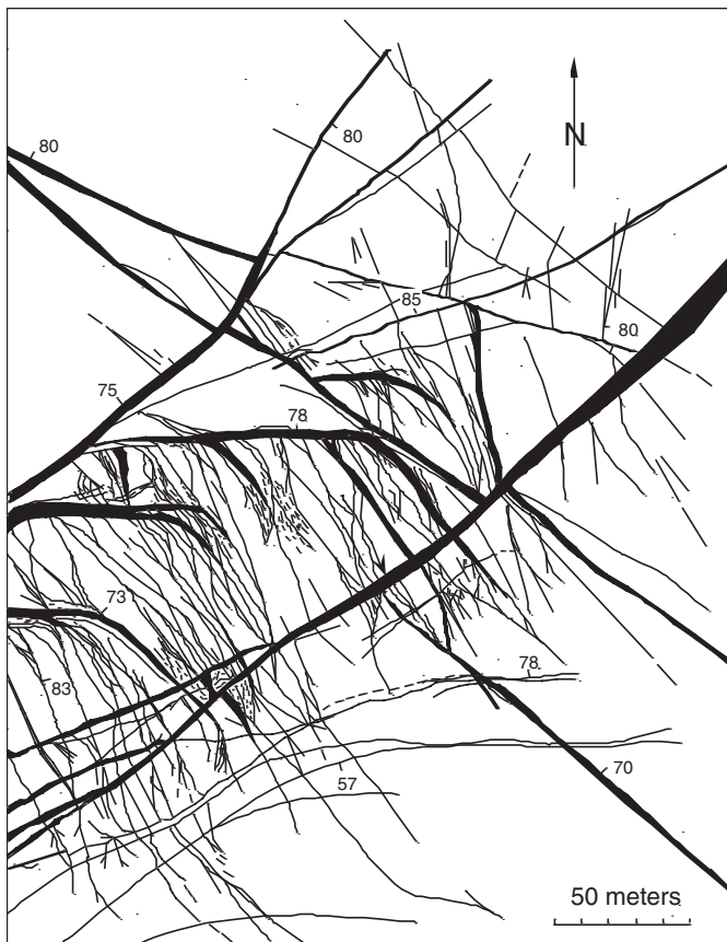
FIG. 25. Fault-related wing-crack arrays associated with fault-controlled mineralization in the Leonard mine, Butte, Montana. Modified after Bateman (1959).
