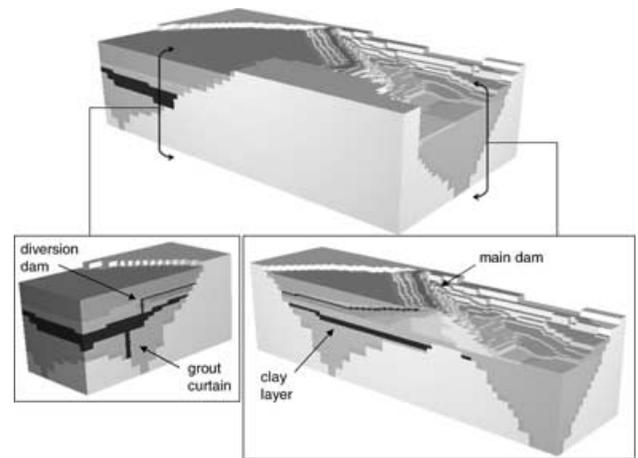
**Figure 16.** Model of the embankment dam and foundation.
