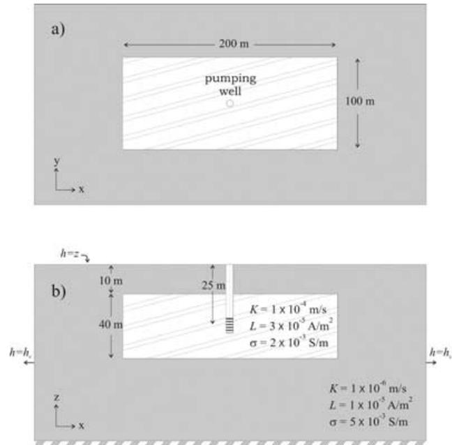
**Figure 10.** Heterogeneous half-space with pumping well: (a) model in plan view, showing outline of subsurface aquifer; (b) model in cross-section, showing hydraulic boundary conditions and physical properties of aquifer and half-space. Well screen length is 10 m.
