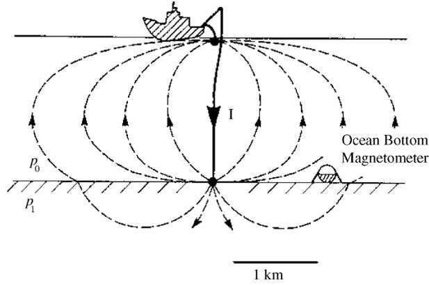
Fig. 2. A schematic of the marine MMR method which shows a vertical bipole source of current and an ocean bottom magnetometer (from Edwards and Nabighian, 1991).
