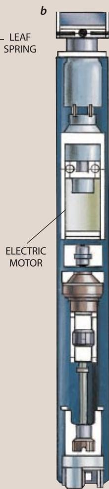
Detail *b* shows the electric motor attached to the tube. This motor spins the cutters against the ice, making chips that are pumped up the outside of the barrel. Such drilling leaves a cylinder, or core, of solid ice inside.
