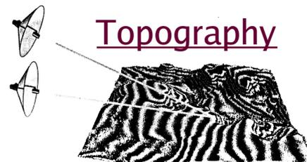
Figure 1.15 Typical interference pattern due to undulating terrain.
