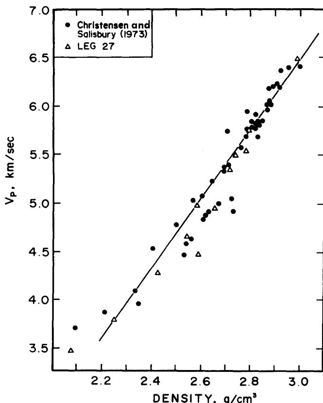
Figure 2. Compressional wave velocities versus densities at 0.5 kb.
