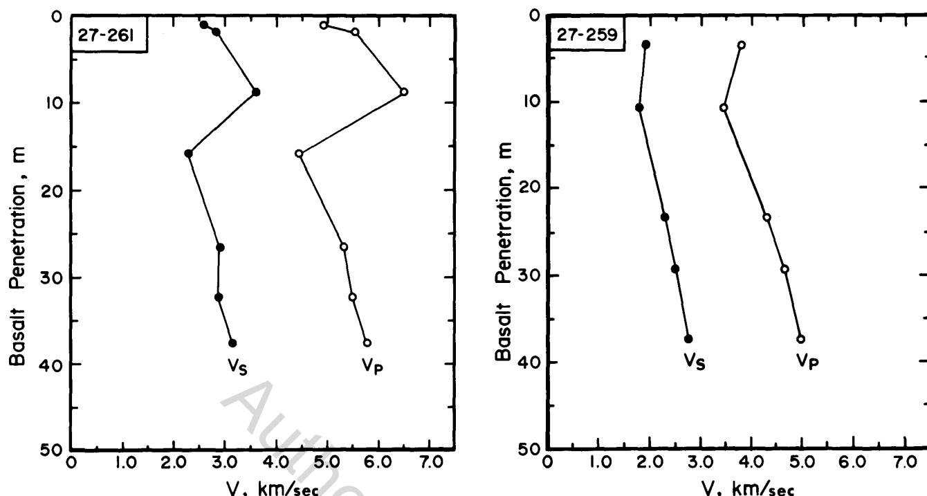
Figure 4. Compressional and shear wave velocities at 0.5 kb versus recovery depth in Layer 2.
