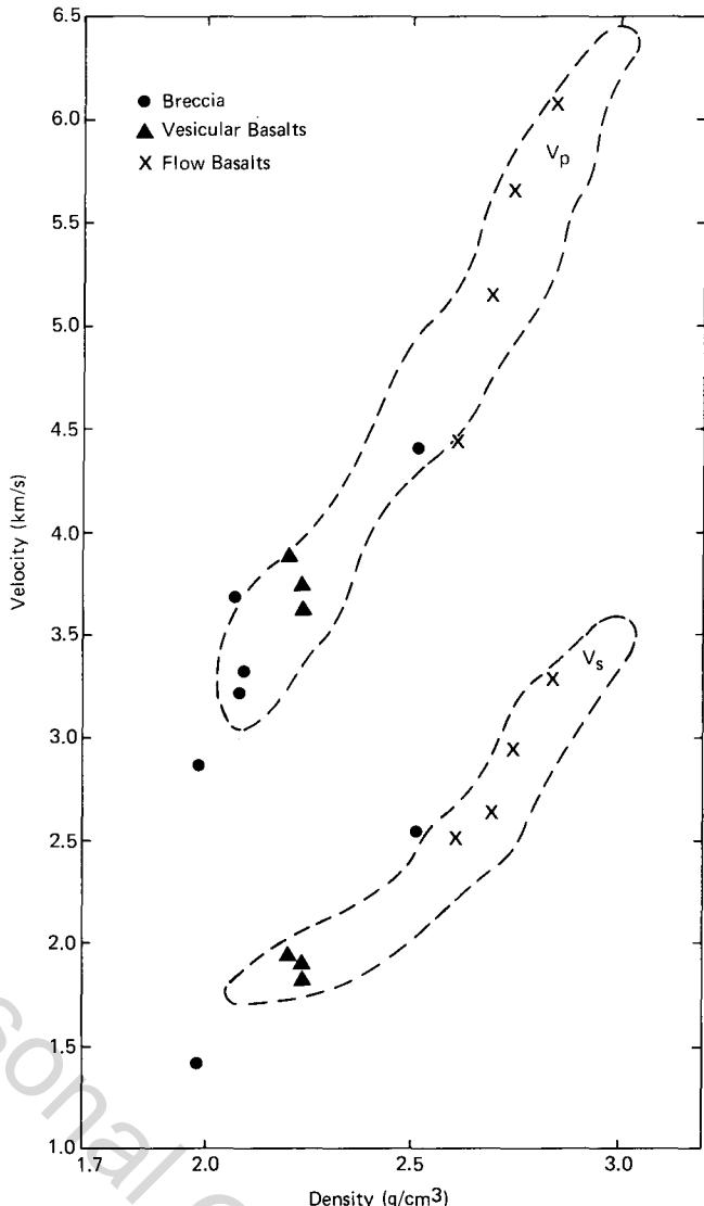
Figure 1. Wet-bulk density versus compressional- and shear-wave velocity at 0.4 kbar for breccias, vesicular basalts, and flow basalts from Leg 59. (Dashed lines enclose previous data for oceanic basalts from Christensen and Salisbury, 1973.)
