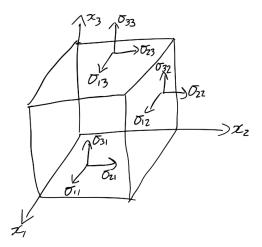
This picture should always be in your head when thinking of elements of the stress tensor.  $\sigma_{ij}$  is the force per unit area in the  $i^{\text{th}}$  direction on the face perpendicular to the  $j^{\text{th}}$  axis.
