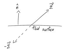
Therefore, if we write Newton's second law of motion  $(\vec{F} = m\vec{a})$  for a volume with a fixed mass of fluid, we have:
