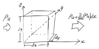
The net mass flux leaving the cube through the face perpendicular to the x-axis with area dy dz is
