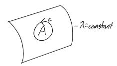
If C is a contour moving with the fluid and if  $\lambda$  is a conserved quantity (which implies that the surface of constant  $\lambda$  also moves with the fluid). Then **the contour** C **remains in the same surface as the fluid moves, for all time**. Recall that Kelvin's theorem says that the equation for the conservation of absolute circulation is (assuming an inviscid fluid):
