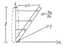
Comparing  $\frac{\Delta\omega_{a,x}}{\omega_a} = \frac{\partial u}{\partial z}\Delta t$  to  $\Delta a = \frac{\partial u}{\partial z}\Delta t l$  shows that  $\frac{\Delta\omega_{a,x}}{\omega_a} = \frac{\Delta x}{l}$ . So the production of vorticity parallel to the x-axis can be interpreted as a simple tilting of the vorticity vector (originally parallel to the z-axis) in the x-direction by the shear.
