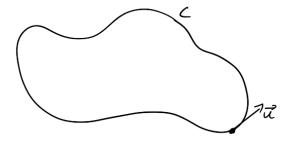
The velocity vector indicates a fluid element on the contour moving with the fluid velocity at that point. One can think of the contour as being composed of a "pearl necklace" of fluid elements (pearls) that moves and deforms in a way defined by the individual motion of the pearls.
