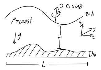
We look for equations that describe the fluid motion in the fluid layer by considering the governing equations and the boundary conditions.
