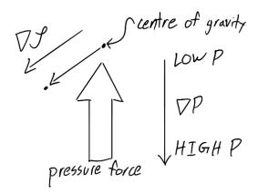
Examining torques around the centre of gravity shows that the fluid will start to spin counter-clockwise, producing positive circulation.
