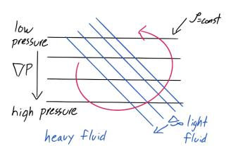
The gradients of the pressure and density fields produce a tendency for the heavy fluid on the left to sink and the light fluids on the right to rise. This induces a positive (counter-clockwise) circulation of the fluid indicated in red.
