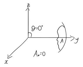
then  $A_n = 0$  and the contribution of planetary vorticity to the vortex tube strength is zero. There is no penetration of A of the lines of vorticity associated with the planetary vorticity.
