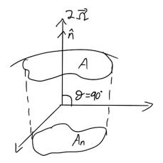
then  $A = A_n$  so the contribution of planetary vorticity to the vortex tube strength is maximum. The penetration of A of the lines of vorticity associated with the planetary vorticity is maximized.
