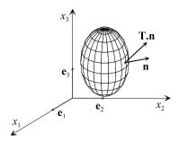
Stress Tensor and Quotient Rule We are given that stress  $T = [T_{ij}]$  at a point x is defined by, see Fig. 1.4,
